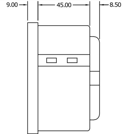
Overall wall thickness 2mm - 2.25mm
